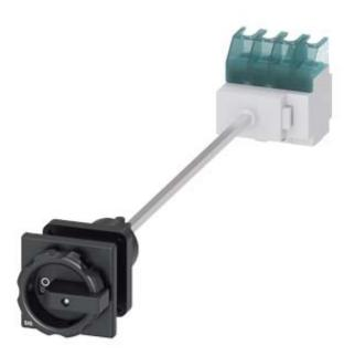
SENTRON, Switch disconnector 3LD, main switch, 4-pole, lu: 25 A, Operating power / at AC-23 A at 400 V: 9.5 kW, floor mounting with door coupling, rotary operating mechanism, black, central mounting 22.5 mm of the handle
