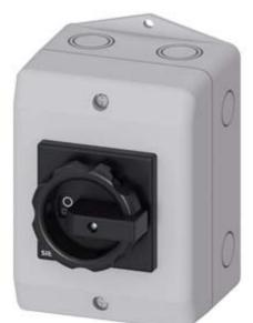
SENTRON, Switch disconnector 3LD, main switch, 4-pole, 16 A, Operating power at AC- 23 A at 400 V: 7.5 kW, molded-plastic encapsulation for metric cable gland, rotary operating mechanism, black
