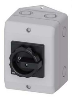
SENTRON, Switch disconnector 3LD, main switch, 3-pole, lu: 16 A, Operating power / at AC-23 A at 400 V: 7.5 kW, molded-plastic encapsulation for inch cable gland, rotary operating mechanism, black
