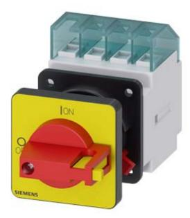
SENTRON, Switch disconnector 3LD, emergency switching-off switch, 3- pole, lu: 16 A, operating power / at AC-23 A 400 V: 7.5 kW, front-mounted, knob-operated mechanism, Red / yellow, central mounting 22.5 mm of the handle
