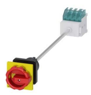
SENTRON, Switch disconnector 3LD, emergency switching-off switch, 3- pole, lu: 16 A, operating power / at AC-23 A 400 V: 7.5 kW, floor mounting with door coupling, rotary operating mechanism, Red / yellow, central mounting 22.5 mm of the handle
