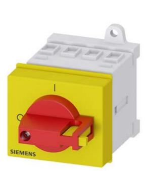
SENTRON, Switch disconnector 3LD, emergency switching-off switch, 4- pole, lu: 16 A, operating power / at AC-23 A 400 V: 7.5 kW, installation in distribution boards, knob-operated mechanism, Red / yellow, handle direct at the switch
