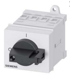
SENTRON, Switch disconnector 3LD, main switch, 3-pole, lu: 16 A, Operating power / at AC-23 A at 400 V: 7.5 kW, installation in distribution boards, knob-operated mechanism, black, handle direct at the switch
