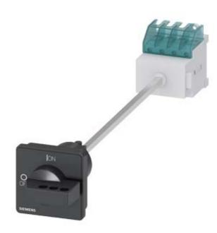
SENTRON, switch disconnector 3LD, main switch, 4-pole, lu: 16 A, operating power / at AC-23 A at 400 V: 7.5 kW, floor mounting with door coupling, defeatable knob-operated mechanism, black, 4-hole mounting of the handle
