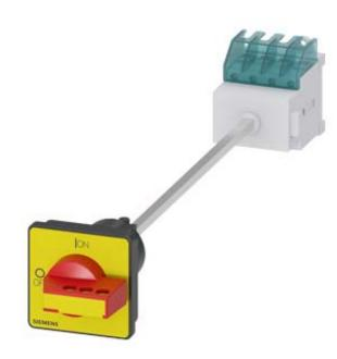
SENTRON, switch disconnector 3LD, EMERGENCY OFF switch, 3pole, lu: 16 A, Operating power / at AC-23 A at 400 V: 7.5 kW, floor mounting with door coupling, defeatable knob-operated mechanism, red/yellow, 4-hole mounting of the handle
