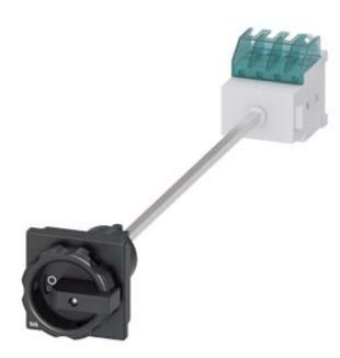
SENTRON, Switch disconnector 3LD, main switch, 3-pole, lu: 16 A, Operating power / at AC-23 A at 400 V: 7.5 kW, floor mounting with door coupling, rotary operating mechanism, black, 4-hole mounting of the handle
