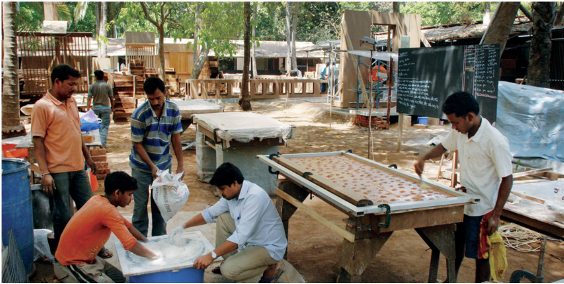
Mezclas de color y moldeado de paneles de escayola para In-Between Architecture Colour mixing and casting of plaster panels for In-Between Architecture Studio Mumbai Workshop, Alibag
