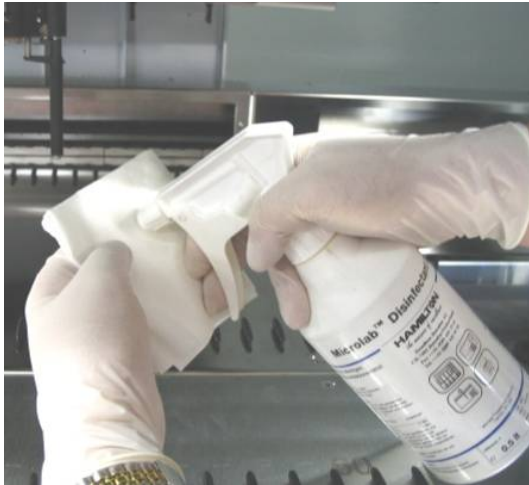
Fig. 41.: Cleaning the Stop Disk and O-Rings
