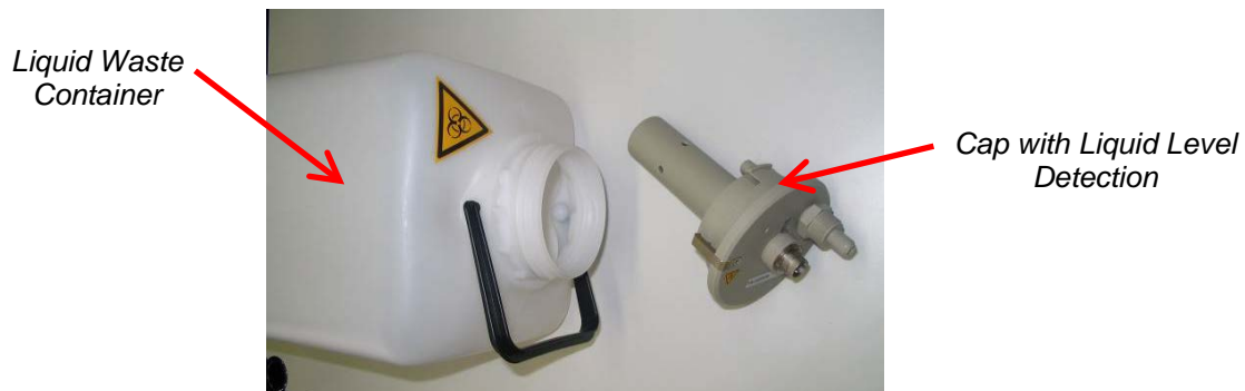
Fig. 5.: Liquid Waste Container and Cap with Liquid Level Detection
