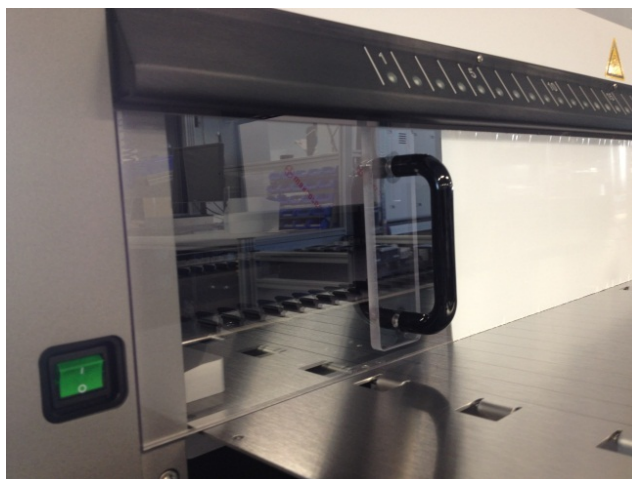
Fig. 43.: Mounting the UV Front Cover
