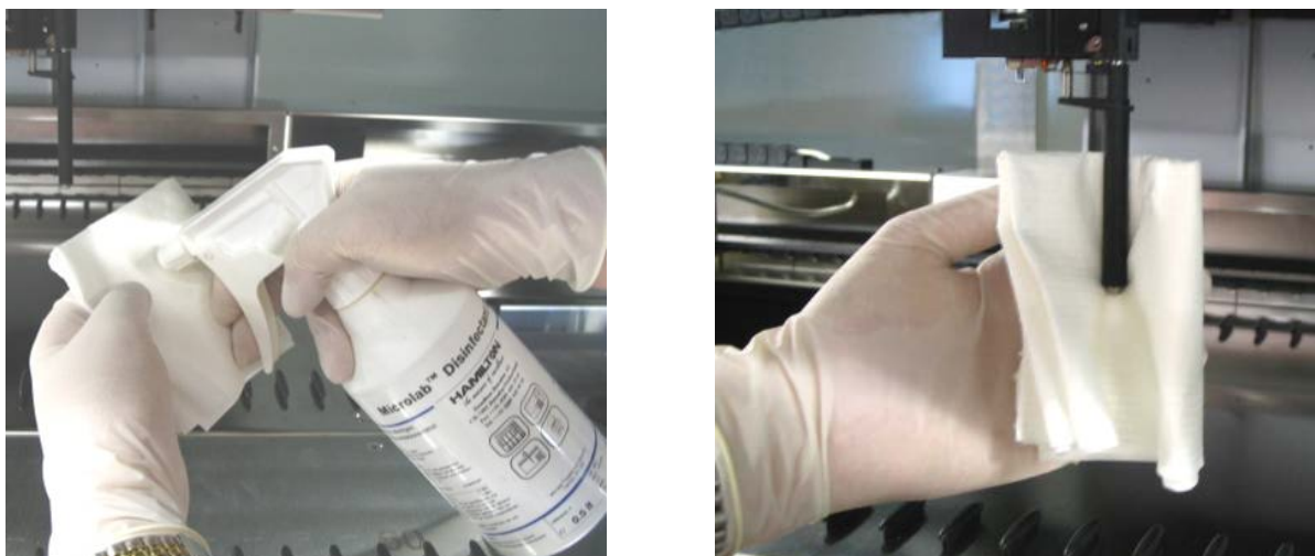
Fig. 40.: Cleaning the Tip Eject Sleeve
