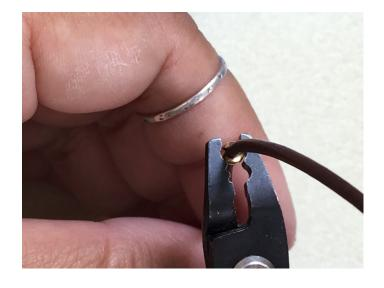
15) In order to close the crimp more tight, use the crimping plier to press against the seam of the crimp cover.
