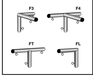
Put the pipe in to the fitting and tighten the screw
