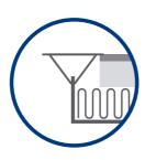
Soundblocker in a spring tee tile. Positioned on top of a Mineral Wool Pad, with the foam facing upwards.
