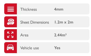
"This is a vinyl sound barrier mat loaded with naturally occurring minerals. The product is free of lead, unrefined aromatic oils and bitumen. Designed to improve the sound insulation of existing panels of metal, wood, plastic etc., at all frequencies."
