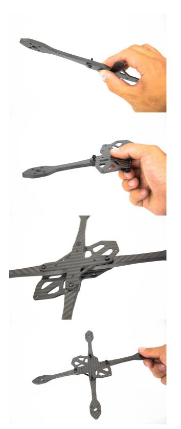
USING A 3X14MM BUTTON HEAD, BOLT THROUGH THE BOTTOM X PLATE AND AN ARM.
