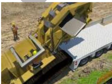
When transportation is required, you will need to drive the machine onto the float. The safest way to do this is to use a spotter to make sure you are moving onto the float as straight as possible and that you stop in the right position to secure the equipment onto the trailer.
