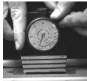
Incorrect alignment of needle to registration mark.
