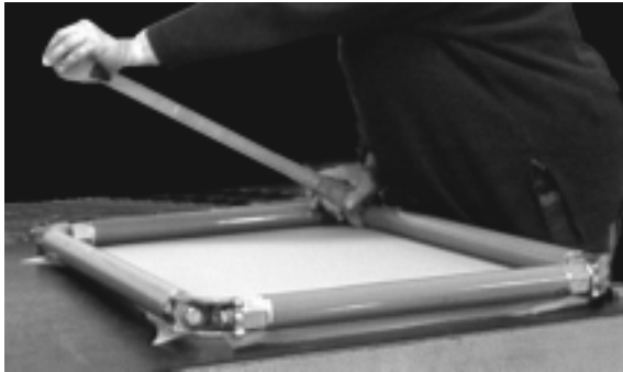
SDI wrench positioned at lowest possible angle.
