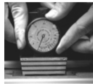
Correct alignment of needle to registration mark.
