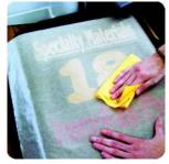
Rub design with pad or chalkboard eraser while still hot to dissipate heat
