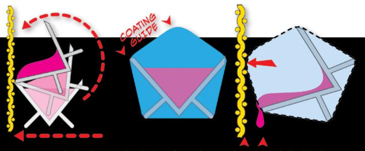
The emulsion will start to flow onto the mesh. Once the emulsion has reached the mesh across the *full length* of the blade of the coater, you can start the coating stroke.
