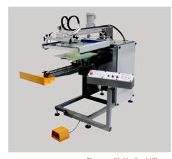
Shown with Vertical Lift, Shuttle Table, and AC Print Head
