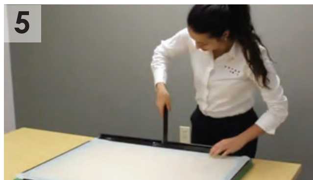
5 Stretch and lock each side in place. You'll hear a nice "snap" when the locking bar is in it's proper position.
