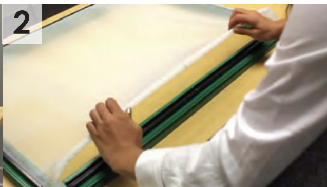
2 Simply snap the panel locking strip into the locking bar channel.
