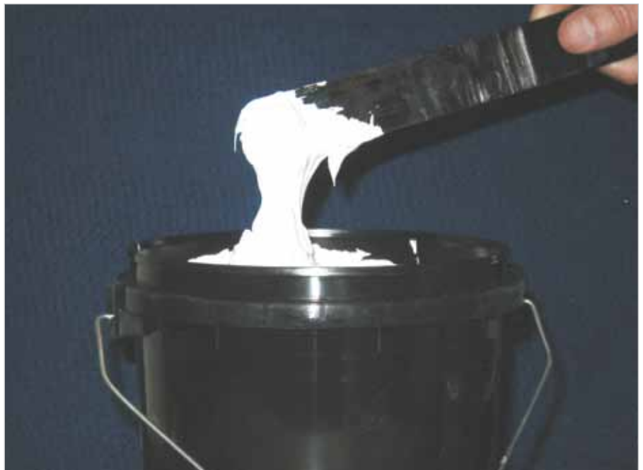
Pigment-rich ink, made for an automatic press: With the metal scoop an inch above the can, a substantial amount of ink is still connected to the source of ink in the can. When printing with an off-contact distance of 1/32", this ink would not shear well from the screen.
