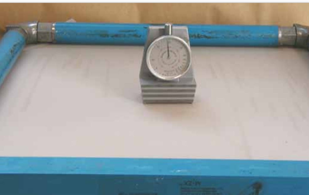
The first variable the author recommends bringing under control in your quest to eliminate or reduce flash curing is that of screen tension. And the most practical way to accomplish that is with retensionable frames.
