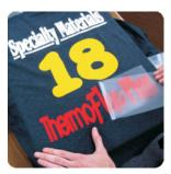
Remove backing after cooling
