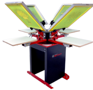
SCOUT 4-Color; 4-Station Rotary Floor Model
