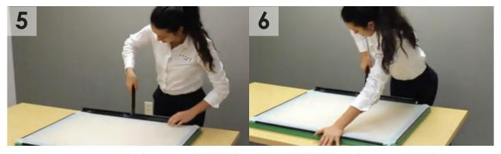
Stretch and lock each side in place. You'll hear a nice "snap" when the locking bar is in it's proper position.
