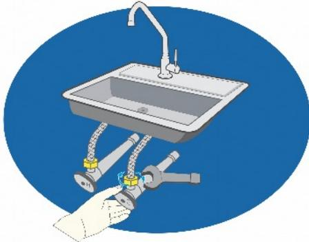
1. Identify the cold water shutoff valve by turning on the faucet cold water, and seeing which shutoff valve makes the water flow stop (usually on the right). Keep the water off during installation.
