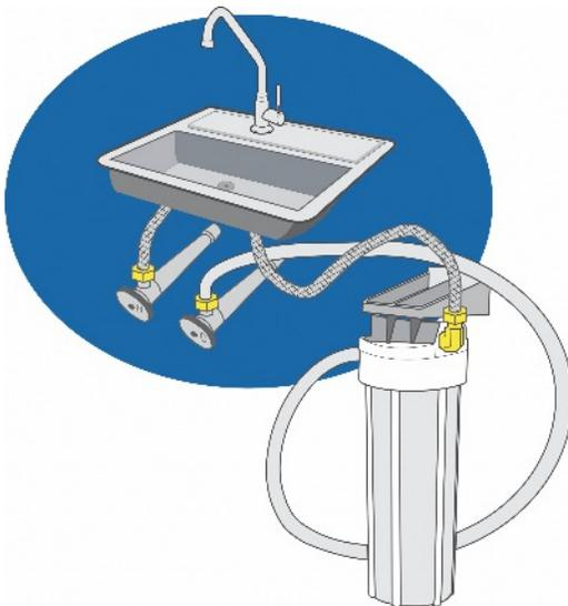
5. Connect the faucet cold water line to the brass fitting on Tailored Tapwater. The nut should be tightened to "finger tight," plus an additional turn with a wrench.
