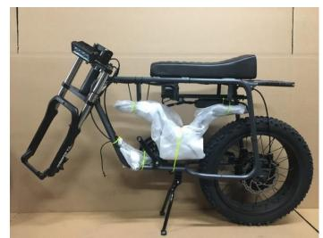
4. Remove the front wheel from its box (this is where that welcome kit is located!), loosen the wheel nuts and slide into drop out. Tighten the wheel nuts using a 15 mm socket wrench and tighten to a torque of 25-30 lb/ft.
