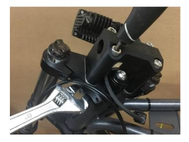
7. Reinstall the riser clamps with the handlebar centered and at desired angle. Make sure the handlebar harness rests between the handlebar risers and below the handlebar. Tighten the riser clamp bolts and coupling nuts to a torque of 15-20 lb/ft.
