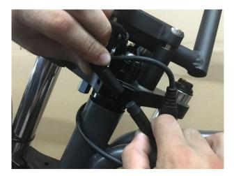
NOTE: CONNECTOR PINS ARE VERY SENSITIVE. LINE UP ARROWS ON MALE AND FEMALE CONECTORS TO ENSURE YOU DO NOT BREAK/DAMAGE PINS.
