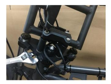
8. Install the brake levers using a 4mm Allen wrench to tighten the clamp bolt. Install the front brake lever on the right side, near the throttle, and the left brake lever on the left side. Route the brake lines in an appropriate manner that eliminates the risk of binding or pulling.
