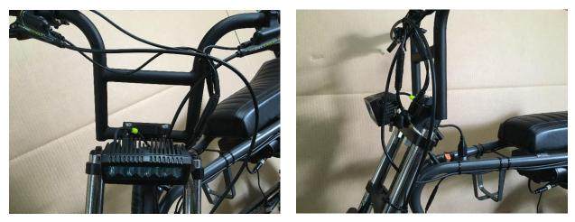
Connect the handlebar harness, and all other connectors, by aligning the alignment arrows stamped on each connector. (RED TO RED, YELLOW TO YELLOW, BLACK TO BLACK) Double-check all connections starting from the motor controller, under battery tray, and following each electrical cable.
