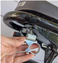
Get them both installed and then slide the mounted tube into the two clamps. This is where you set the angle of the mounted tube as well.
