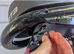
We need to reconfigure some parts in the box. Open up the front mount, disassemble, and pull out the two tube clamps (right photo below)
