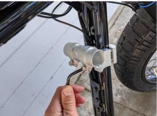
Out Back we're going to install using the two outer mounting holes of the rear light bracket. Locate and remove them.
