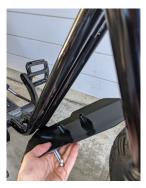
Install the Clamp as high as you can, in the orientation shown. Tighten the bolts evenly. Adjust the angle of the mounted tube with the tube clamp bolts as shown on the right.
