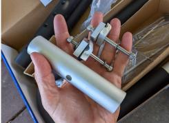
Combine and assemble as shown here. Then you are ready to screw them into the threaded holes of the frame where we took the bolts out. If you happen to have a drill, drilling out the holes in the rack clamps will make this step go smoother, but it's not necessary.
