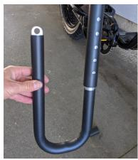
On the rear bar, if you have a light, it makes it a little hard to access the push button on the bars. It is easy to switch the button direction to make it easier to access the button. Pop the cap with a knife and fish out the button with a bent piece or wire (coat hanger will do)
