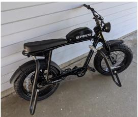
Set Bar Height: On this demo bike, the height of the rear bar is about perfect, but the front bar is a little too low. Cut some foam off the front bar to raise it up slightly
