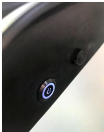
To turn off the power, press the button again and it will pop back up and return to the flush position.
