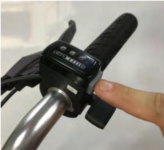
Dis-engage the kickstand. Do not sit on bike with kickstand engaged. Seat yourself on the Super73. Activate power by pressing on the power button on the throttle mount. Make sure the battery button is on.
