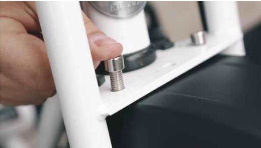
Slide one of the bigger bolts through the hole on the triple tree so that it goes all the way through to the underside of the fender.
