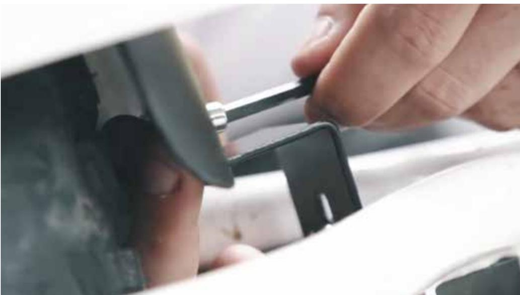
Use a 4mm Allen key to tighten the bolt to the point where you can still move it for final adjustments.
