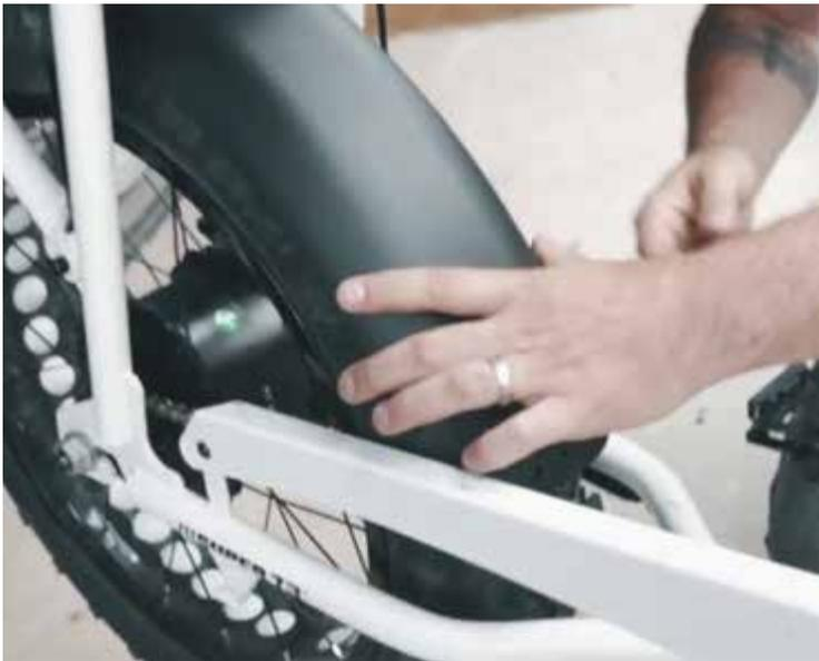
Take the rear fender with the two holes facing the front of the bike and put it on top of the tire.
