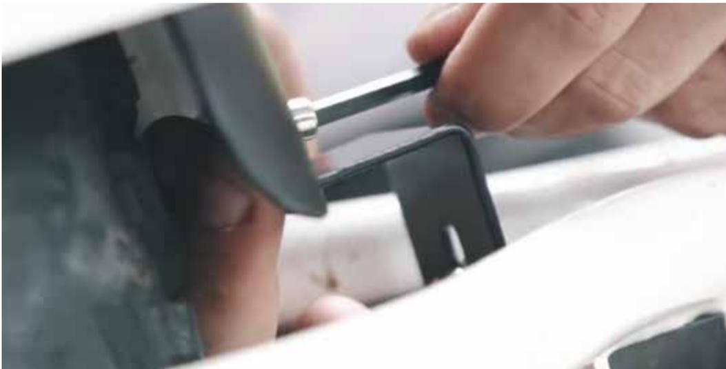
Put the bolt through both the center bracket and rear fender. Take the lock nut and place it on the back of the bolts and hand thread them in.
