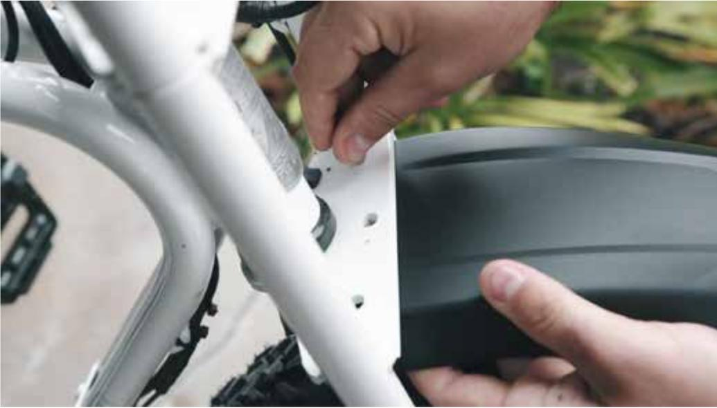
Place front fender underneath the front fork of the bike and line up the 3 holes of the fender with the 3 holes on the triple tree.
