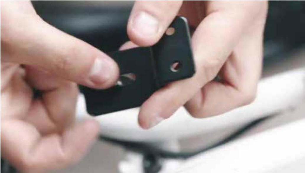
Find the front bracket and one of the small bolts. Slide through the rear of long slot.
