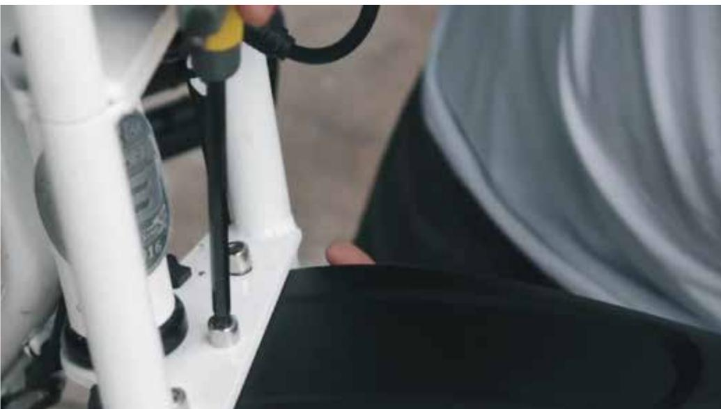
Take the washer and nut and align them on the bottom side of the fender.
