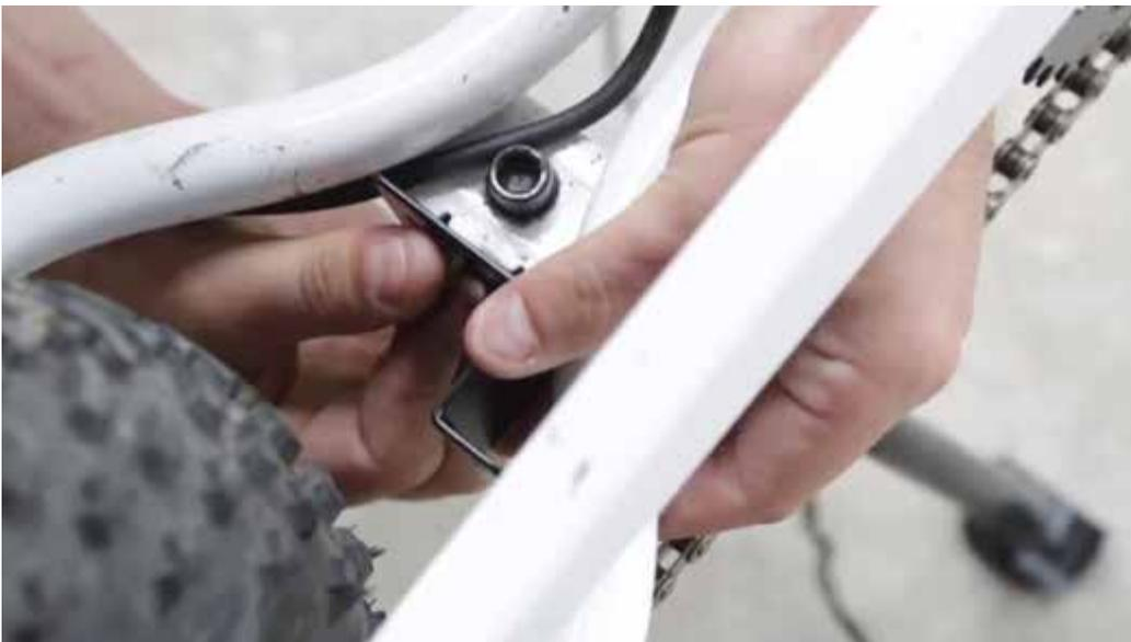
Hand tighten the bolt into the accessory mount located at the bottom of the frame in front of the rear wheel.
