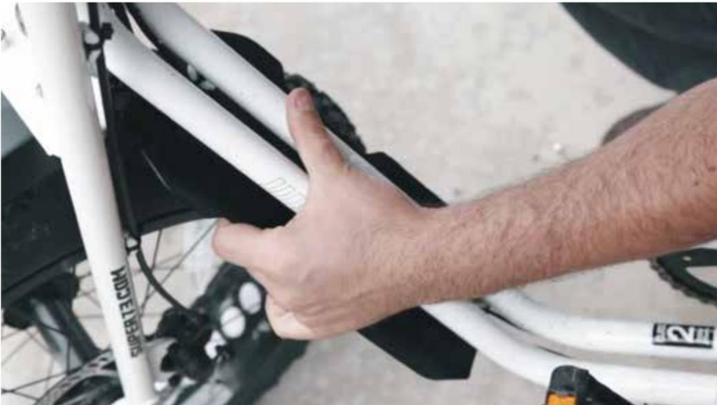
Place the guard against the frame. Make sure that the front wheel still has proper clearance when it turns and that none of the cables are hindering the guard from lying flat against the frame.
