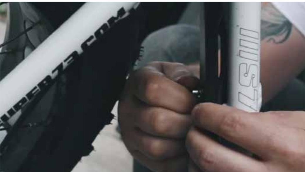
Push one of the long screws with the washer through the sleeve of the splash guard first and begin to hand thread the screw into the accessory mount on the frame.
