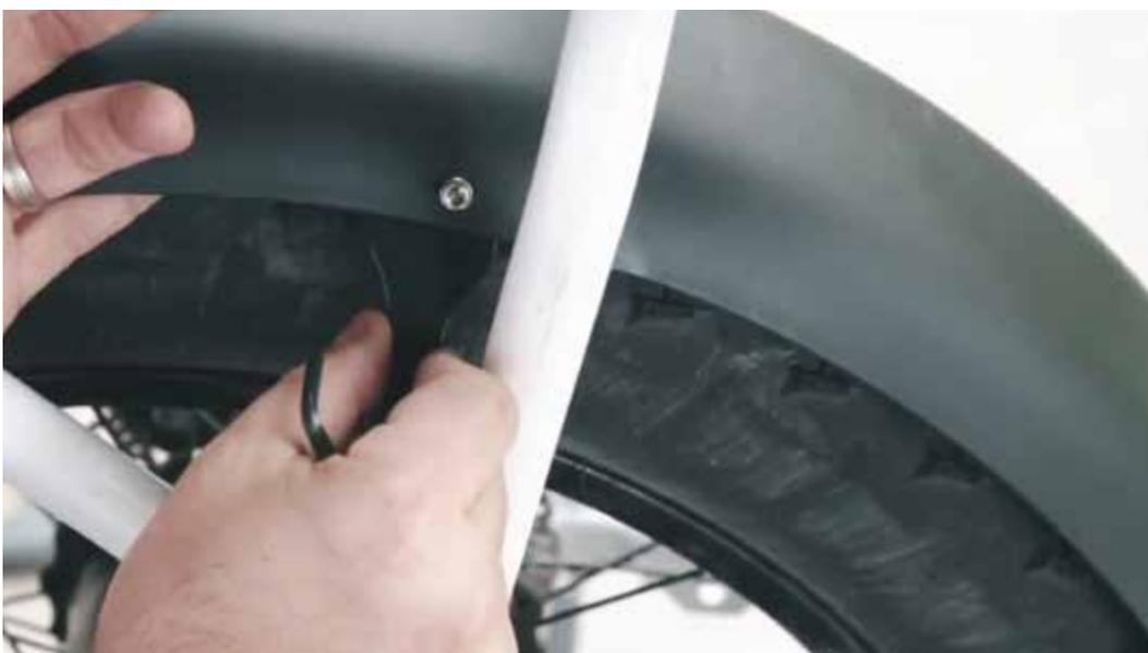
Place the fender over the top of the rear bracket and line up the holes to push your bolt through both the fender holes and rear bracket. Adjust bracket and place nut on the back side of the bolt. Repeat last step for the other side.
