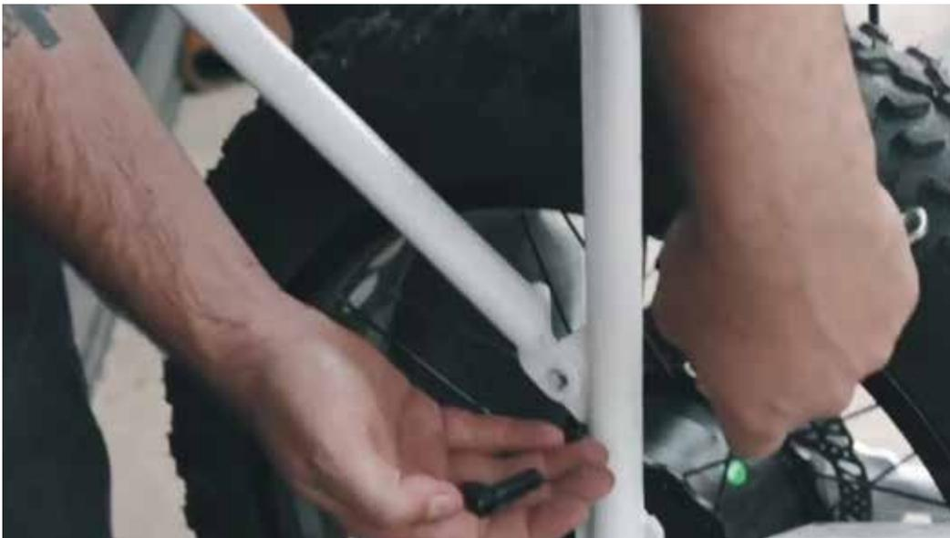
Begin by removing the bolts for your rear rack using the adjustable wrench and 6mm allen key
