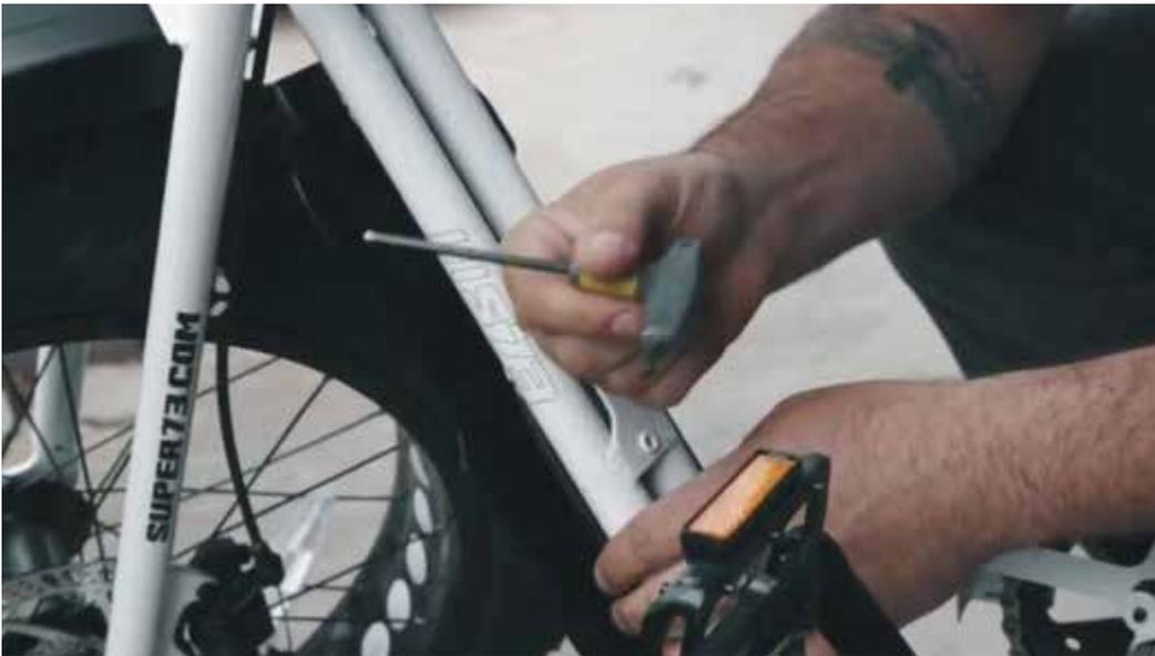
Use a 4 mm allen key to fully tighten down the screws.
