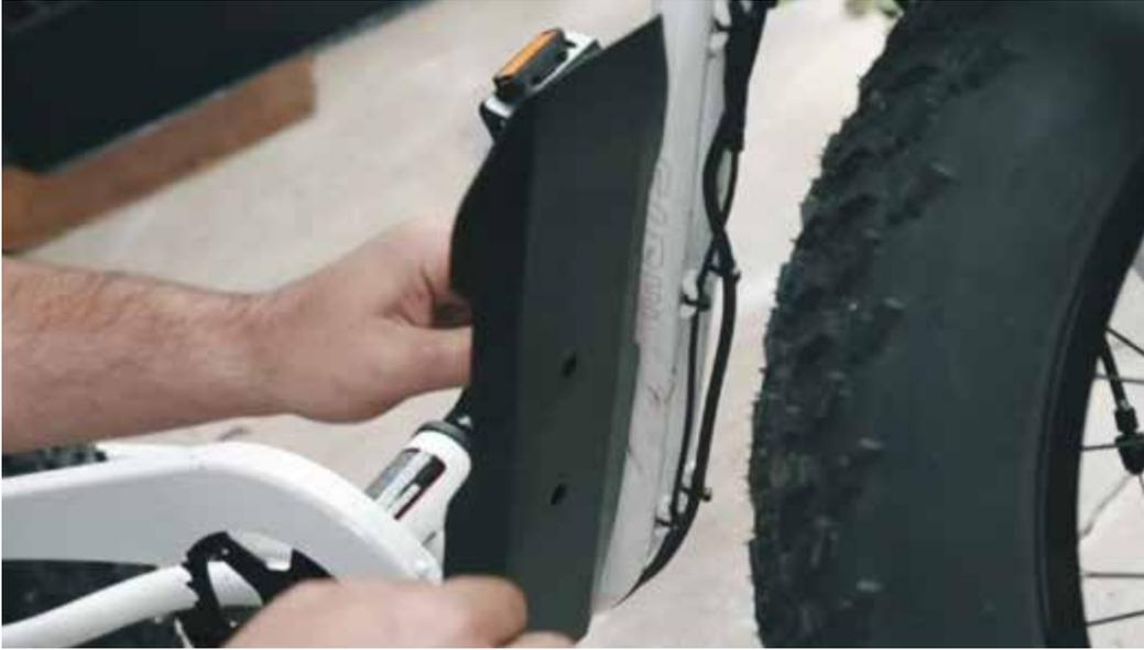
Make sure the side cutouts of the splash guard are on the top side when you align the sleeves on the splash guard with the accessory mounts located on the frame directly behind the front wheel.
