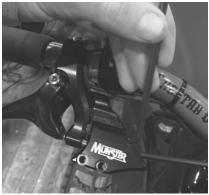
(3) Install the two 6mm bolts from the packaging of your throttle guard into the throttle guard body to fasten it to the finger throttle. Tighten the bolts so that the throttle guard body is mated fully and secure.
