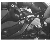
(4) Install the lever guard onto the guard body the same way you took it apart. Before you tighten the bolts fully, you can slide the lever side to side to adjust for rider preference. Tighten the bolts fully, making sure not to over tighten them and strip the threads.
