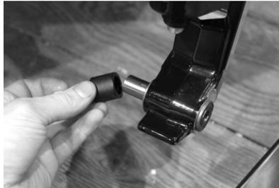
(4) Remove the plastic spacer from the sleeve. Save the plastic spacer in case you want to return it back to stock when you sell your snowmobile. Install one of your new ski bushing savers in place of the plastic spacer. The ski bushing savers can be mounted on either side of the spindle to make your ski stance wide or narrow depending on rider preference.
