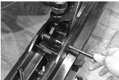
(2) Remove the bolt from the ski to take the ski off of the spindle. You may have to pull hard and turn the bolt to get it out.
