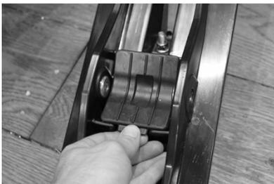
(3) Inspect the ski bushing for damage. Replace the ski bushing if necessary.
