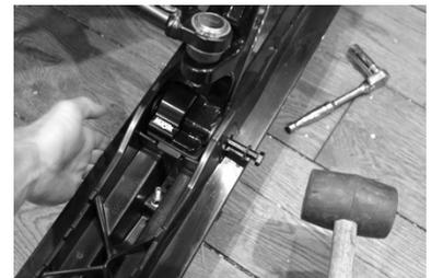
(6) Once the ski bolt is in place, install and tighten the nut.
