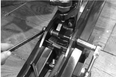
(1) Lift up the front of your snowmobile and set it on a block to suspend the skis off the ground. Using a 15mm and 16mm wrench, undo one of the bolts holding the skis to the spindles.
