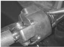
(13) With a torx screw driver remove the 4 screws from the back of the throttle assembly.
