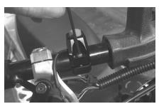
Remove the clamp from the Munster reverse switch with an Alan key and install the switch on the handle bar in your desired position.
