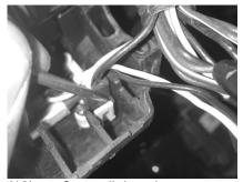
(18) Once all the wires are exposed, disconnect the plug connector to your reverse switch. If you are installing a Munster kill switch, disconnect the plug connector to the kill switch as well. (See kill switch instructions for pictures and further information)
