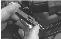
Plug the reverse switch connector into the appropriate matching plug on the machine. You may want to slice the wiring harness casing holding the reverse switch wires to relocate them, depending where you mounted the switch. Use zip ties to secure the wiring harness and any loose wiring.
