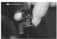
(5) Pull the needle tool towards the pin connector to pry the locking mechanism inside the plug away from the pin connector. At the same time, pull on the individual wire you are trying to release. You may want to get someone to help you for this step. If done correctly, the wire should pull out easily. If the wire is pulled before you pry back the locking mechanism the pin connector will not release.
