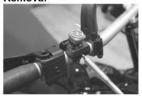
(1) Unscrew the small torx screw to remove the stock kill switch assembly.
