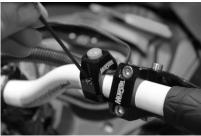
(6) Remove the clamp from the Munster kill switch with an Alan key and install the kill switch on the handle bar in your desired location. Route the kill switch wires through the wiring harness.
