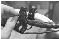
(8) Use zip ties to secure the wiring harness. Re-install the riser cover and you're done!
