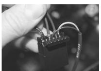
(7) Plug the pin connectors for the kill switch into the plug in any order, but make sure to orient the pins in the right direction. Once they are fully seated and clipped in, flip the plug locking mechanism closed. Plug the connector plug back into the wiring harness.
