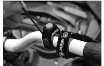
(6) Remove the clamp from the Munster kill switch with an Alan key and install the kill switch on the handle bar in your desired location. Route the kill switch wires through the wiring harness.
