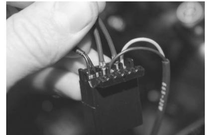
(7) Plug the pin connectors for the kill switch into the plug in any order, but make sure to orient the pins in the right direction. Once they are fully seated and clipped in, flip the plug locking mechanism closed. Plug the connector plug back into the wiring harness.
