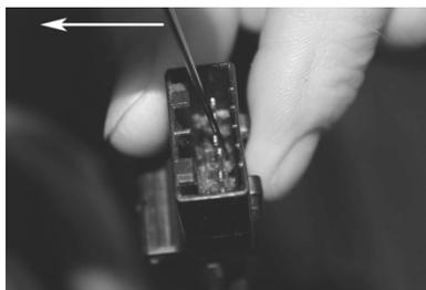
(5) Pull the needle tool towards the pin connector to pry the locking mechanism inside the plug away from the pin connector. At the same time, pull on the individual wire you are trying to release. You may want to get someone to help you for this step. If done correctly, the wire should pull out easily. If the wire is pulled before you pry back the locking mechanism the pin connector will not release.
