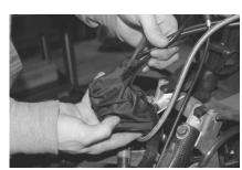
(6) With your new kill switch connected, cover up the harness plugs with the cloth boot and tuck
