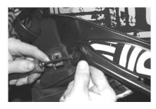
(3) Take off both side panels of your machine. Using a small flat head screwdriver release the two rivet tabs on either side of the hood by prying the centers out. Slide the hood forward to release it. Undo all wire harness plugs connected to the hood to properly remove the hood from the machine.
