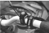
(7) Remove the clamp from the Munster kill switch with an Alan key. Install the kill switch on the handle bar in your desired position, routing the wires appropriately.
