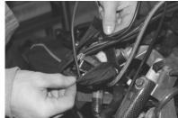
(4) Pull out the black cloth cover that contains the wiring harness tucked in front of the steering column. Undo the Velcro to expose the wire plugs.
