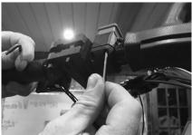
(13) With a torx screw driver remove the 4 screws from the back of the kill switch assembly.Remove the assembly from the handle bar.
