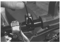
Remove the clamp from the Munster kill switch with an alan key and install the switch on the handle bar in your desired position.
