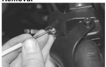
(1) Use a small screwdriver to remove the E-clip holding the throttle cable housing in place. Pull the cable housing out and slide the cable through the slot to detach the housing.
