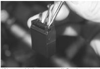
(5) Using a small flat head screwdriver release the small clips on the plug and flip the locking tab back to expose the pin connectors in the plug.
