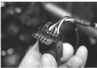
(9) Locate the wires coming from the thumb heater. Repeat step 6 to remove all thumb heater wires from the plug.
