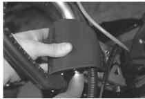
(17) Reinstall the riser cover making sure all wires are routed in their original location.
