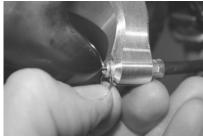
(14) Using the low profile C-clip provided with your finger throttle, install it over the end of the cable housing to secure it in place.
