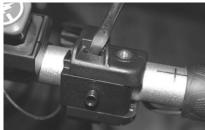
(3) Using an Alan key, undo the bolt on the clamping plate of the thumb throttle. Use a flat head screwdriver to push in the small tab while sliding the plastic clamping plate away from your grip. (Some models may have different style throttle block) You may have to take off the kill switch by removing the torx screw before
