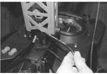
(11) Re-route the throttle cable through your riser so it can be installed in front of the handlebars. Keep in mind the cable must be clear of the riser cover when it is installed later. Make sure the cable housing is away from any pinch points. Check your steering for full range of motion making sure it doesn't put any tension or stress on your throttle cable housing.
