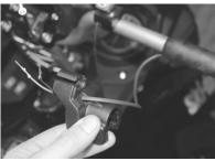
(8) Remembering which wires go where, repeat step 6 to remove the other grip heater wire(s) going to the plug. Once the grip heater wire(s) are free from the plug remove the throttle block, pulling the grip heater wires through the hole in the block. Reinsert the grip heater pin connectors into the plug in their original location.
