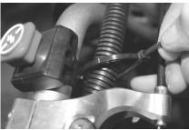
(16) Tuck all heater and kill switch wires back together and use zip ties to fasten to the handle bar.
