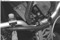
(4) Take off the riser cover to expose the wiring harness plugs. Follow the wires from the thumb heater and the right hand grip heater to the wiring harness, cutting the zip ties to expose the wires. Unplug the harness plug that the wires go to.
