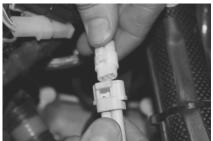
(13) Plug the white jumper connector provided with your finger throttle into the throttle safety switch plug.
