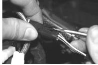
(11) Follow the wires from your thumb heater to the harness plug and disconnect the plug by prying up the locking tab with a screwdriver.
