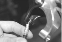
(15) After routing the throttle cable in front of the handlebars, insert the throttle cable end into the finger lever slot.
