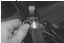
(22) Adjust finger throttle for rider preference. Tighten clamp bolts, and you're done!
