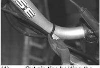
(4) Cut zip ties holding the wires running from the throttle block to the handlebars.
