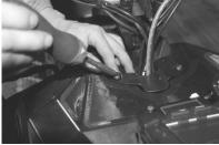
(2) Undo the two bolts around the steering column holding the hood on and slide the hood forward to release it. Undo all wire harness plugs connected to the hood to properly remove the hood from the machine.
