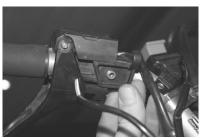
(6) With the backing plate off, undo the bolt on the clamping plate of the thumb throttle and slide it away from your grip to remove it.
