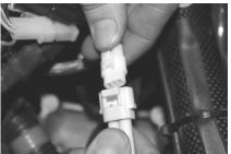
(13) Plug the white jumper connector provided with your finger throttle into the plug the throttle position switch was disconnected from.
