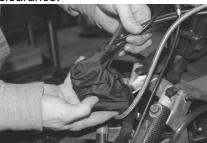
(20) Cover up the harness plugs with the cloth boot and tuck them back into the machine. Put the hood back on making sure to connect all the harness plugs that were disconnected earlier. Fasten hood bolts and rivets. Install side panels.
