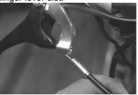
(16) Pull on the cable housing. Slide the cable through the slot in the aluminum block and release the housing into place.
