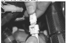
(10) Follow the wires from the throttle position switch to the harness plug. Using your thumb, press down the lock tab to disconnect the plug connector.
