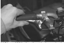
(19) With the throttle lever in the full throttle position, tighten the cable
