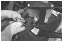
(3) Slide the pivot bolt out from the assembly and remove the rubber boot and brake lever.
