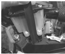
(2) Using a strong piece of tape, slide it between where the brake lever contacts the piston in the master cylinder to hold the piston from falling out when you remove the lever. Make sure the tape is pulled tight and fastened well against the master cylinder.
