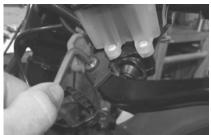
1) Loosen off the torx pivot bolt on the stock brake lever, but do not remove it yet from the assembly.
