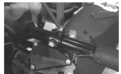
(9) Loosen the master cylinder clamp bolts and position the brake assembly for rider preference. Re-tighten clamp bolts. Apply and release the brake several times, as well as test the park brake to make sure everything is functioning properly. If the brake feels spongy and/or the piston in the master cylinder leaked or fell out at any point during the install, the brakes will need to be bled to insure no air is in the brake lines. Refer to your owner's manual for this procedure.
