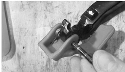
(5) Remove the pin from the park brake assembly, being careful not lose the spring when you take it apart.
