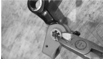
(4) With the brake lever off, cut the small retaining clip holding the park brake assembly together on the lever.
