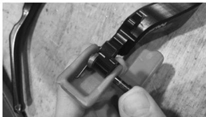
(6) Assemble the park brake lever and spring on to the Munster brake lever with the handle of the red park brake lever facing the logo side of the Munster brake lever, and the spring on the opposite side as shown in the picture. Make sure one end of the spring is inserted in the small hole of the red lever and the other end is bracing against the brake lever. Slide the pin in from the top down through both levers and spring.
