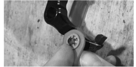
(7) Locate the small retaining clip included with the Munster brake lever. Slide the clip firmly over the end of the pin to hold the park brake assembly in place.
