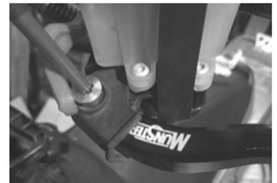
(8) Slide the rubber boot on to the brake lever and install the lever on to the brake assembly. Install and tighten the pivot bolt, and remove the tape you applied earlier holding the piston in the master cylinder.
