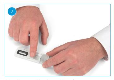
When the sample has been collected, the test administrator slides the tamper-proof cover across the Cartridge to secure the sample.
