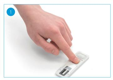
The fingerprint sample is collected by firmly pressing all ten fingertips in sequence onto the Intelligent Fingerprinting Cartridge sample pad for five seconds each.
