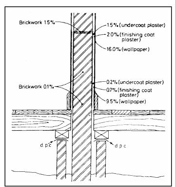
Concentration of salts in a party wall in which rising damp has persisted for 80 years. The figures show the percentage by weight of chloride plus nitrate. The shaded area is heavily contaminated.(Redrawn from Building Research Establishment Digest 245. revised 1987)
