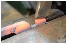
**2.** Heat the jaw end and use a hot chisel to split the jaw about <sup>1</sup>/<sub>4</sub>" down.
