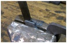
1. Heat the ends of the Quick Bolt Tong blanks. Clamp in a vise and split using a sharp hot chisel
