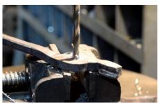
**6.** Mark the center of the hinge area and drill a <sup>1</sup>/<sub>4</sub>" hole.
