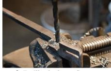
**6.** Drill a hole to fit your rivet.
