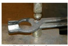
**4.** Drill a hole to fit your rivet and rivet both blanks together.
