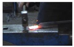
3. Shape the jaw on the anvil. (For flat jaw tongs, the jaw can be left as is, but I prefer to thin the end a little, makes grabbing a piece out of the fire easier.)
