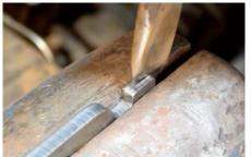
1. Use a hot chisel to make a groove down the center of the jaw of each tong.
