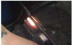
Tong jaws can also be shaped under a power hammer. Here, I am using a 1" bottom swage and a ½" round rod to form the jaw.
