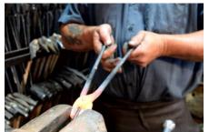
**9.** Make final adjustments on the tongs by heating and squeezing reins to ensure they are lined up properly and will be comfortable to hold on to.
