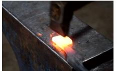
1. Use a cross peen hammer to thin the jaw of each tong blank to about 1/8".
