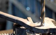
**5.** Mark the center of the hinge area and drill a ¼" hole. If desired, draw out and/or sand the edges of the reins.
