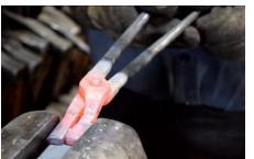
**8.** Make final adjustments by heating and squeezing/twisting as necessary to ensure the reins are lined up properly and will be comfortable to hold on to.
