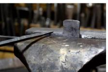
**2.** Insert one blank into the vise with the reins to the left and the inside of the jaw lined up with the top of the vise and hammer back 90 degrees. This will become your left blank. To do the right blank, insert into the vise with the reins to the right, line up the same way, and hammer back 90 degrees.
