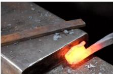
3. Use the step of the anvil to bend the U-shape into the jaw for both the right and left blank.
