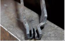
**4.** Put an offset in the jaw area of the right and left blank using the edge of the anvil and light blows. (See video for more detailed instructions)
