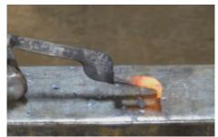
4. Shape the jaw on the edge of the anvil to thin and curl the end.
